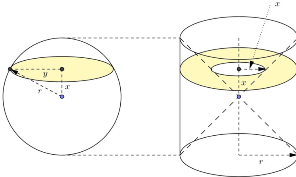
In the diagrams we have a sphere on the left and, on the right, a cylinder with two cones cut out (which meet in the point shown in the very centre of the cylinder). Note that the sphere of diameter  $2r$  would fit perfectly inside the cylinder of height  $2r$ .
